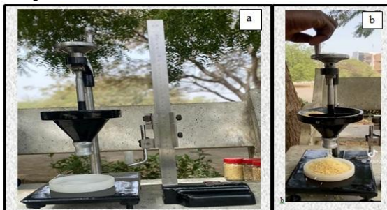
(a) Full view of the Apparatus; (b) Testing the AOR of rice grain
