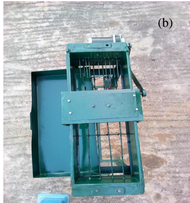
Fig 1. (a) Isometric View of Cucumber Slicing Machine; (b) Constructed Cucumber Slicing Machine.
