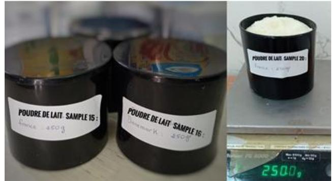
Fig 1. Samples conditioning in Marinelli Beakers
