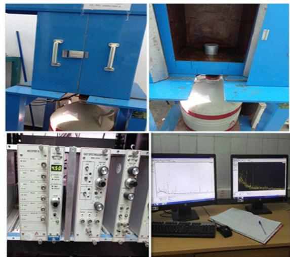
Fig 2. Gamma spectrometry system
