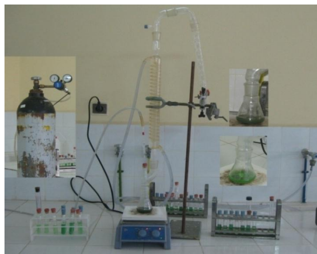
Fig 3. Experimental device used for dissolving of uranium oxides under inert atmosphere.
