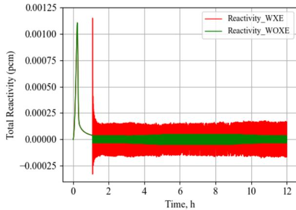
Fig 8. Total reactivity in reactor core (unfiltered signal).
