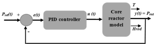
Fig 1. Reactor core power control strategy with PID controller.
