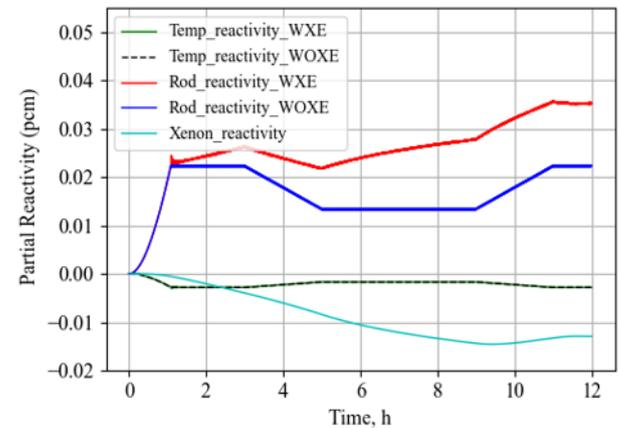
Fig 7. Partial reactivity due to rod movement, coolant temperature, and xenon.
