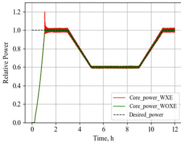
Fig 3. Power variation with PID controller [100%-60%-100%].
